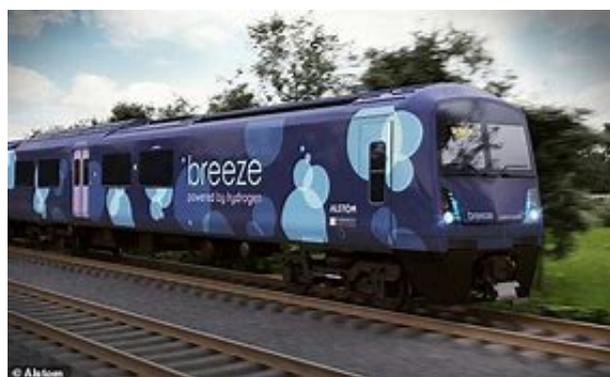
**The proposed appearance of the converted Class 321 multiple unit. Gauge restriction in the UK means that hydrogen cells will be located within the body structure of the vehicle rather than on the roof as in Europe**
