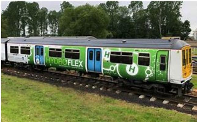
**Main line certification is to be progressed for the Porterbrook / Birmingham University HydroFLEX Class 319 multiple unit conversion illustrated above after a successful period of test track running**
