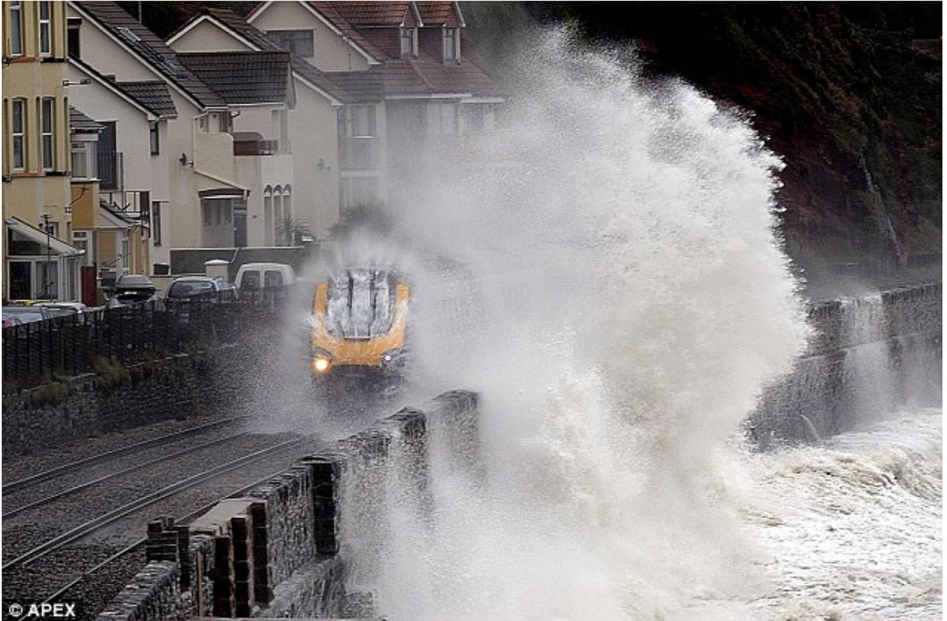
Class 220 Voyager trains have roof mounted electrical equipment which is prone to failure when encountering the type of operating conditions illustrated on the West Country route
