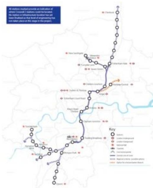
Crossrail 2 is a £27.5 billion project to connect existing rail routes in south-west and north-east London with a 36 kilometres central section of twin tunnels that will link Wimbledon and Tottenham Hale/New Southgate.
